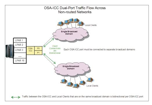
Figure 45. Network topology Diagram 1
