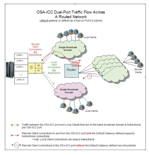
Figure 1. Network topology diagram
