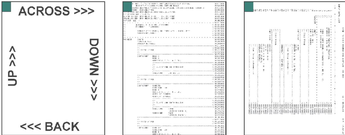
Figure 148. Fixed Media Origins for the IBM 3820 Printer
