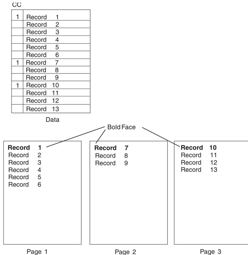
Figure 32. Font Change Using FONT Commands and Subcommands
