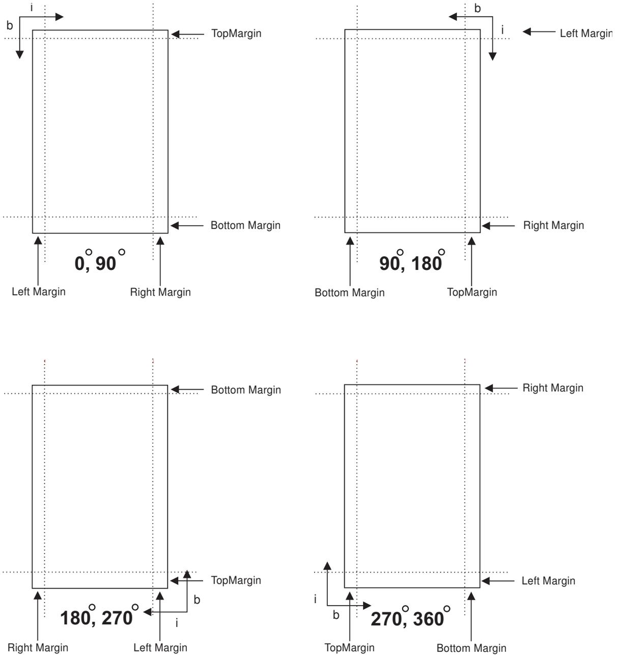
Figure 45. Relationship of Margin Definition to Text Orientation
