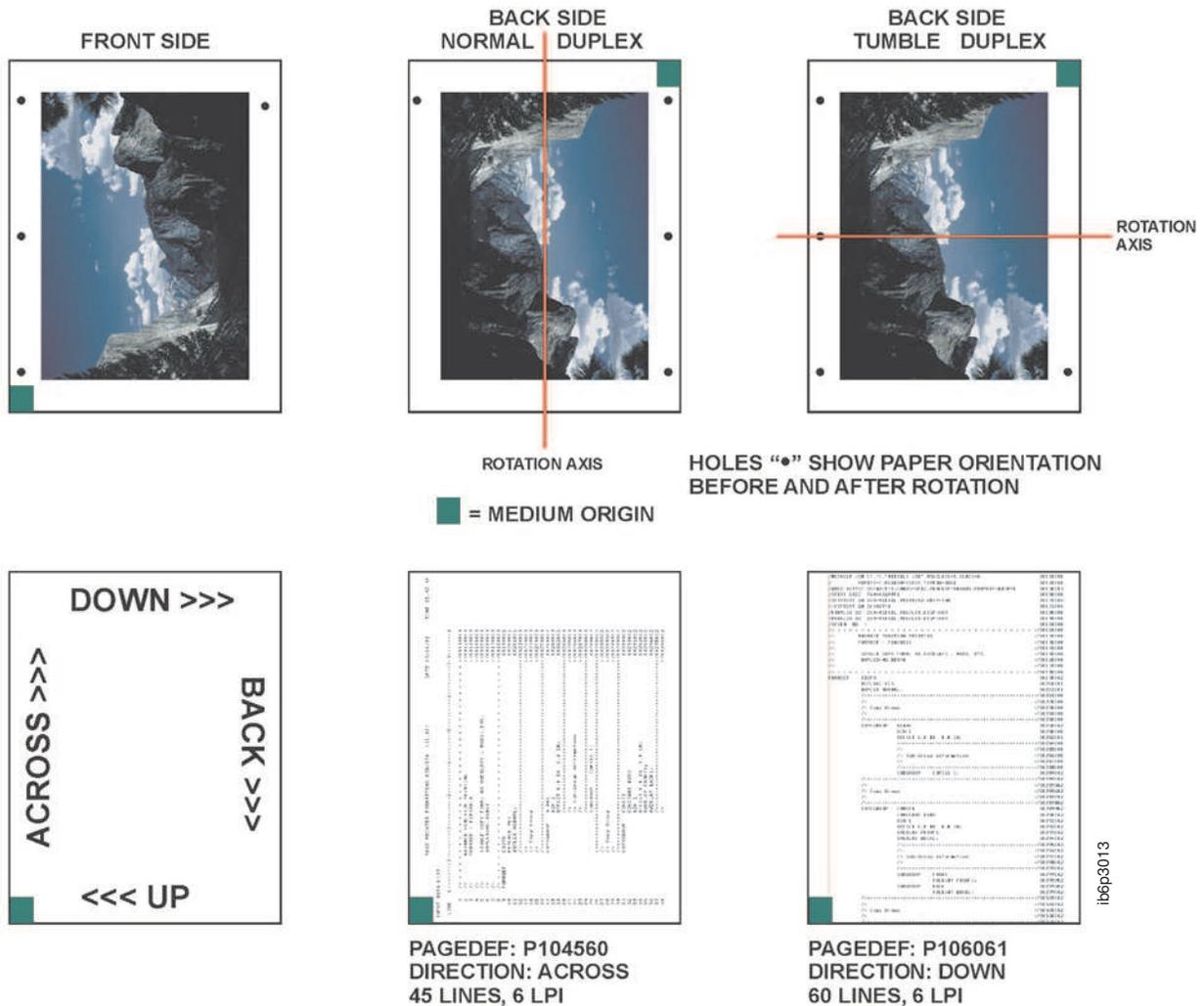
Figure 154. Cut-Sheet Printer with a Medium Origin of X'04'
