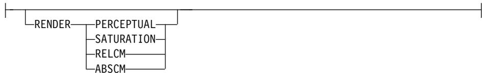
Subcommand on the DRAWGRAPHIC command that is used to specify the rendering intent (RI) for an object within a page definition. RI is used to modify the final appearance of color data and is defined by the International Color Consortium (ICC). For more information about RI, see the current level of the ICC Specification.
