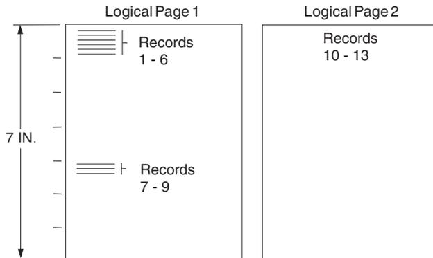
Figure 26. Printout Example Specifying POSITION MARGIN TOP and POSITION MARGIN 4.1
