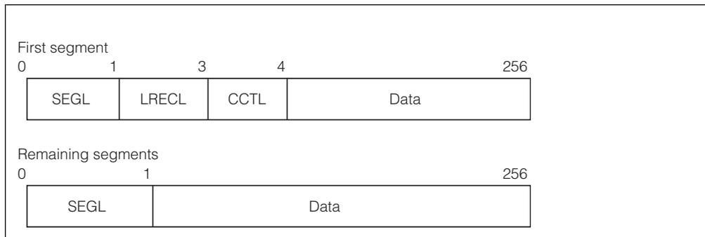
Figure 23. Spanned Data Record With Carriage Control
