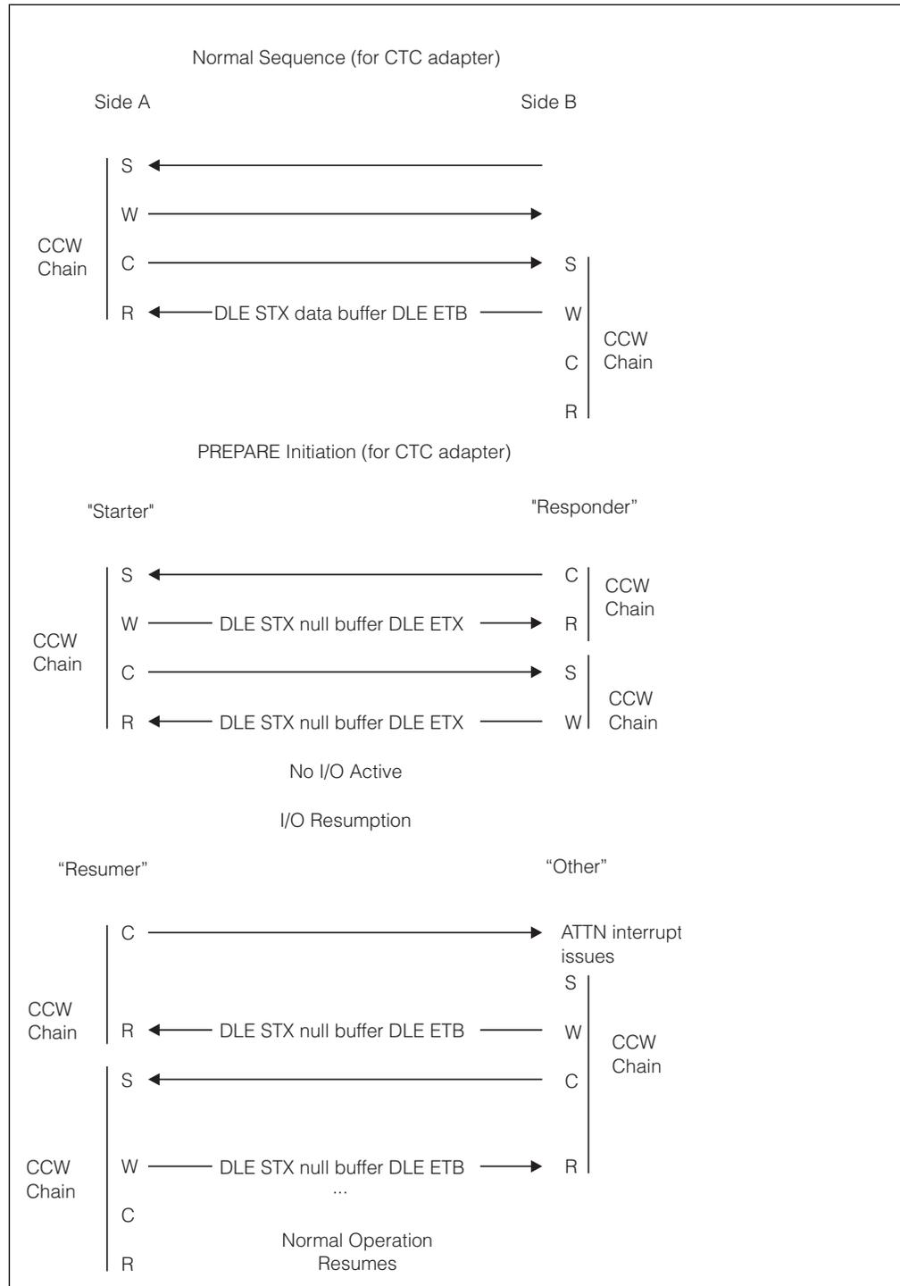
Figure 46. CTC Adapter Communication Procedure Shown Graphically
