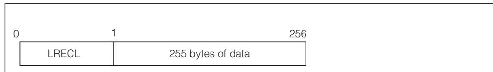
Figure 20. Data Record Without Carriage Control
