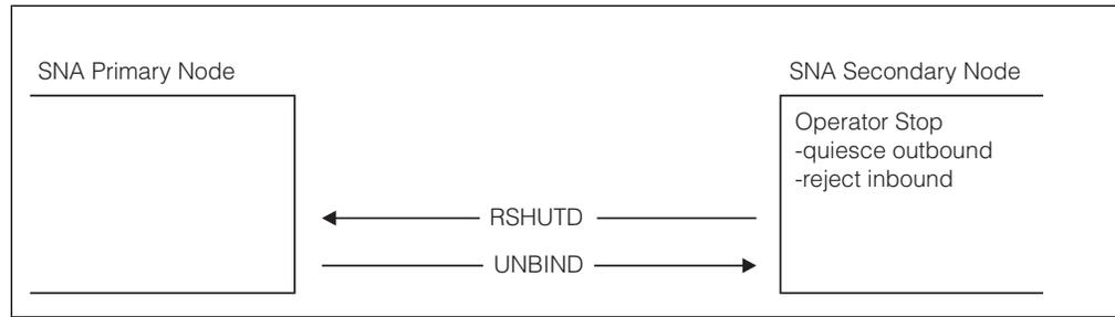
Figure 13. Terminating Processing by an SNA Secondary Node
