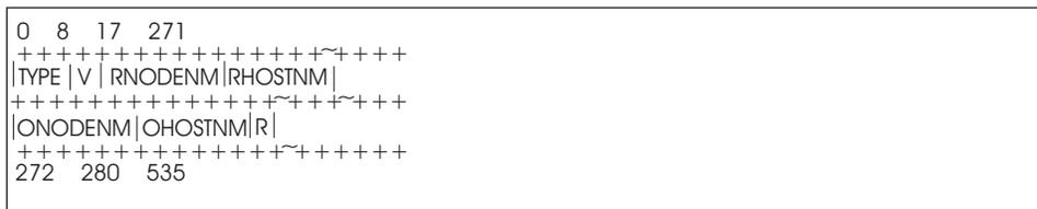
Figure 62. Format of an IPV6 NJE Control Record
