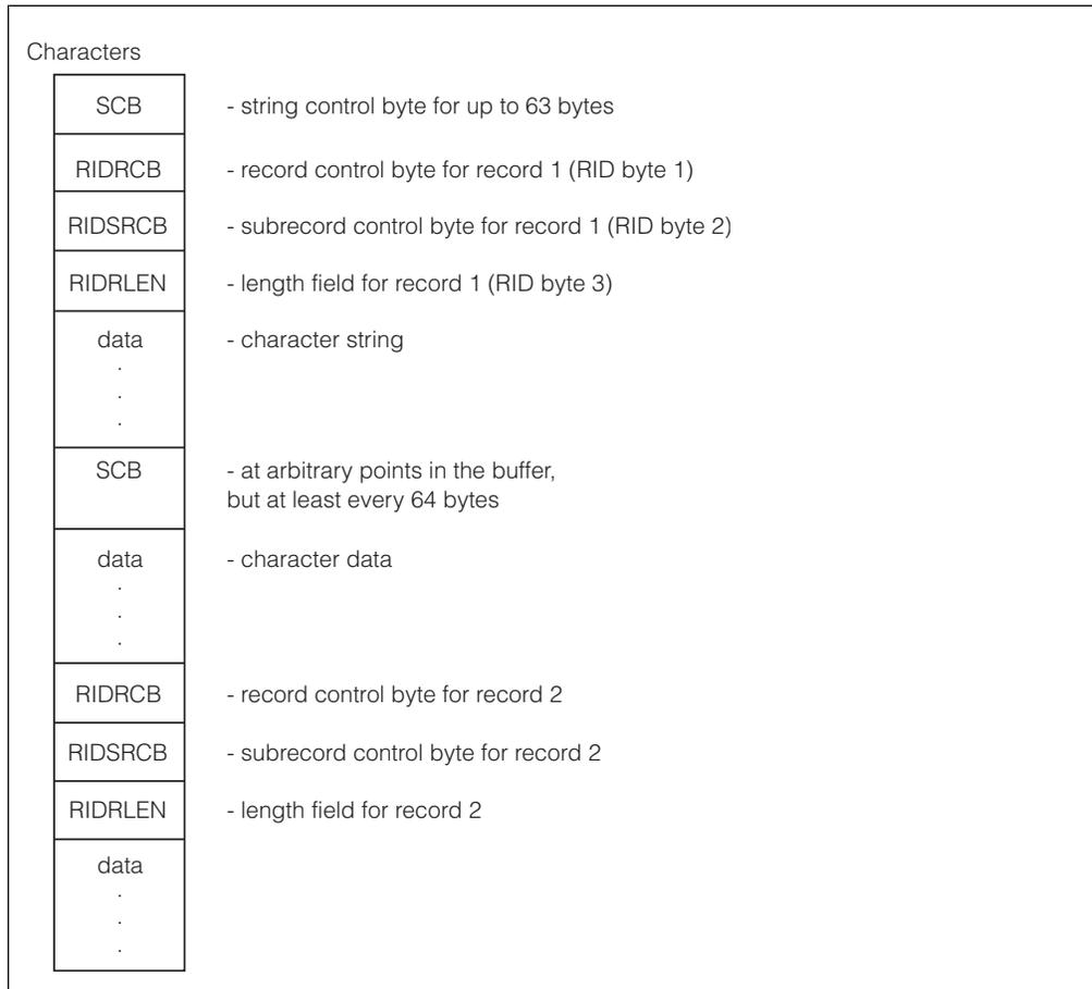
Figure 19. Format of a Transmission Buffer for SNA
