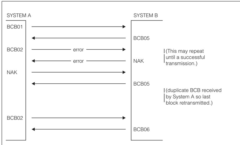
Figure 17. Correct Recovery with Null Records
