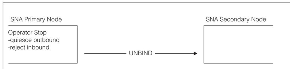
Figure 14. Terminating Processing by an SNA Primary Node
