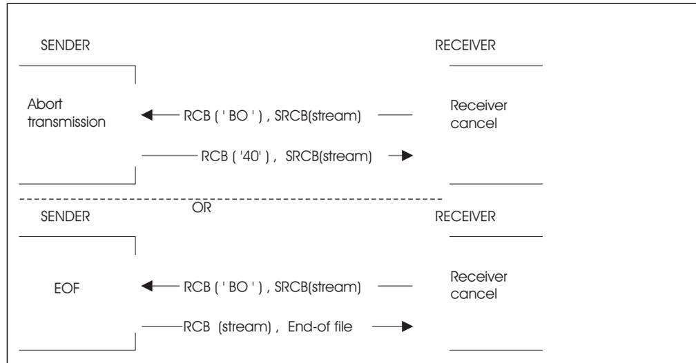
Figure 27. Receiving Node Initiates Stream End
