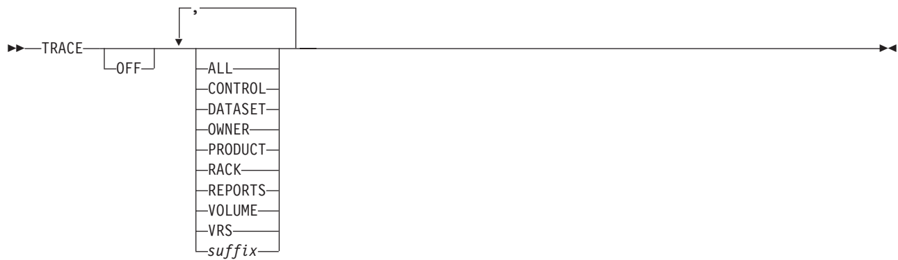
Figure 4. TRACE command syntax diagram
