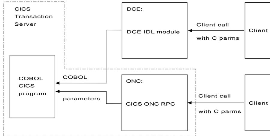
Figure 5. Remote procedures provided for DCE RPC and ONC RPC
