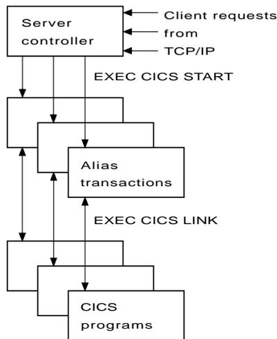
Figure 47. The server controller and alias transactions
