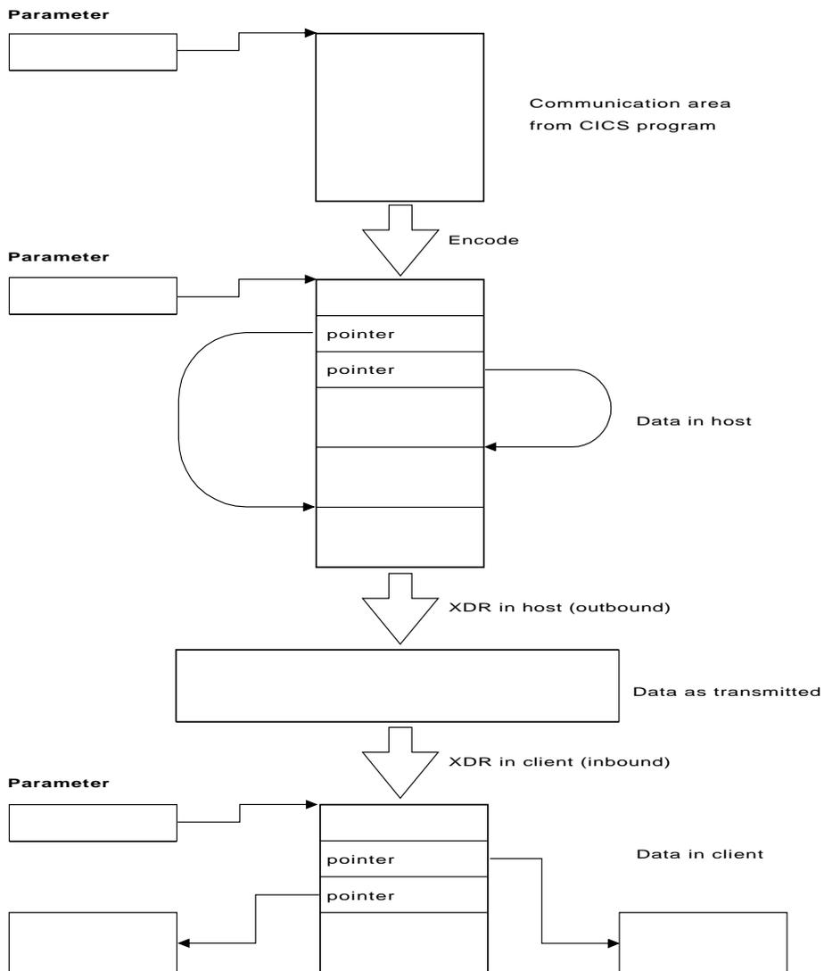
Figure 51. Data flow from CICS program to client
