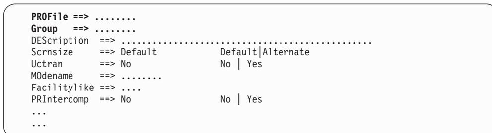
Figure 16. The DEFINE panel for the PROFILE resource definition
