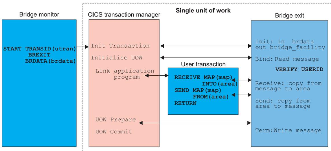
Figure 9. A simple terminal transaction
