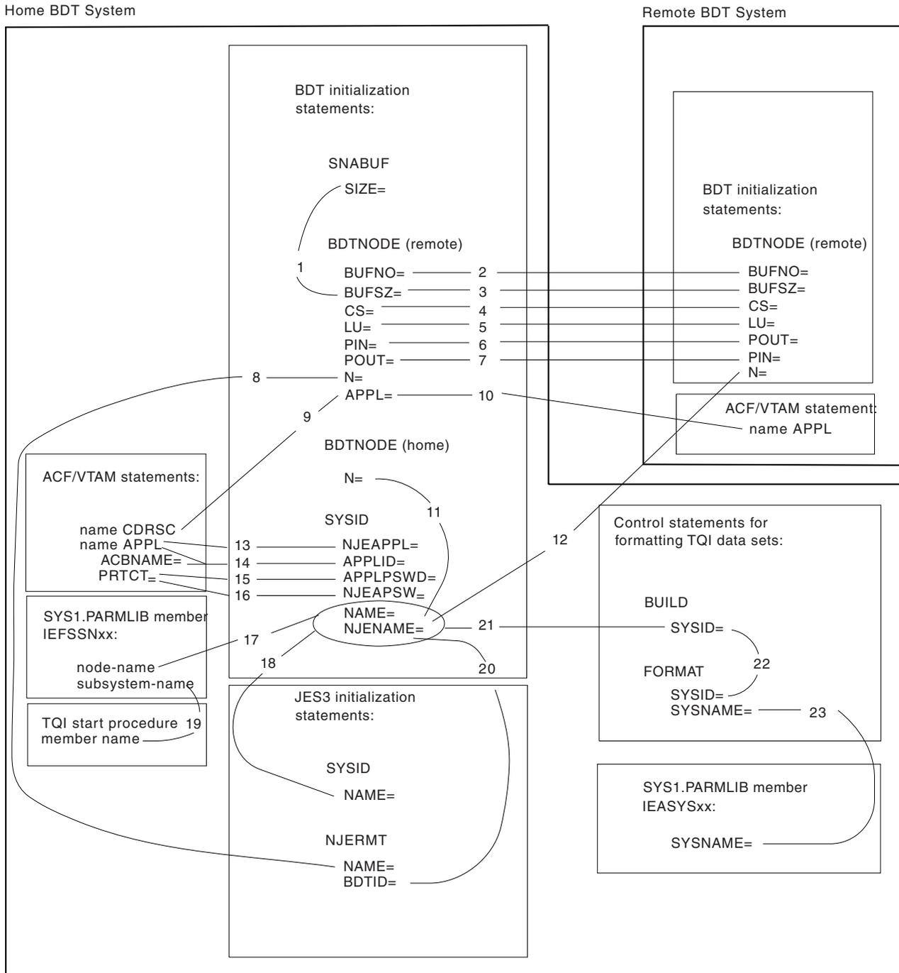
Figure 31. Matchups between BDT, MVS, and VTAM parameters. The numbers in the figure are keys to the explanations that follow.
