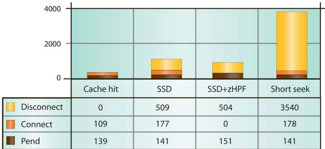
Figure 3: High Performance FICON and SSD technology to reduce I/O service times
